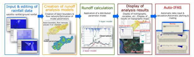
Figure 2-1 Calculation flow of IFAS
