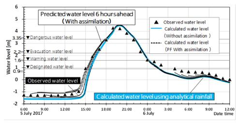
Example of the assimilation of water-level data using the Particle Kalman Filter method
