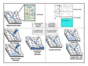
Schematic diagram of the WEB-RRI model based on the water and energy budget and four main modules: 1. Calculation of the water and energy budget between the atmosphere and the land surface in each model grid; 2. Vertical soil moisture distribution calculation; 3.
