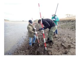
Sediment size survey in a downstream area
