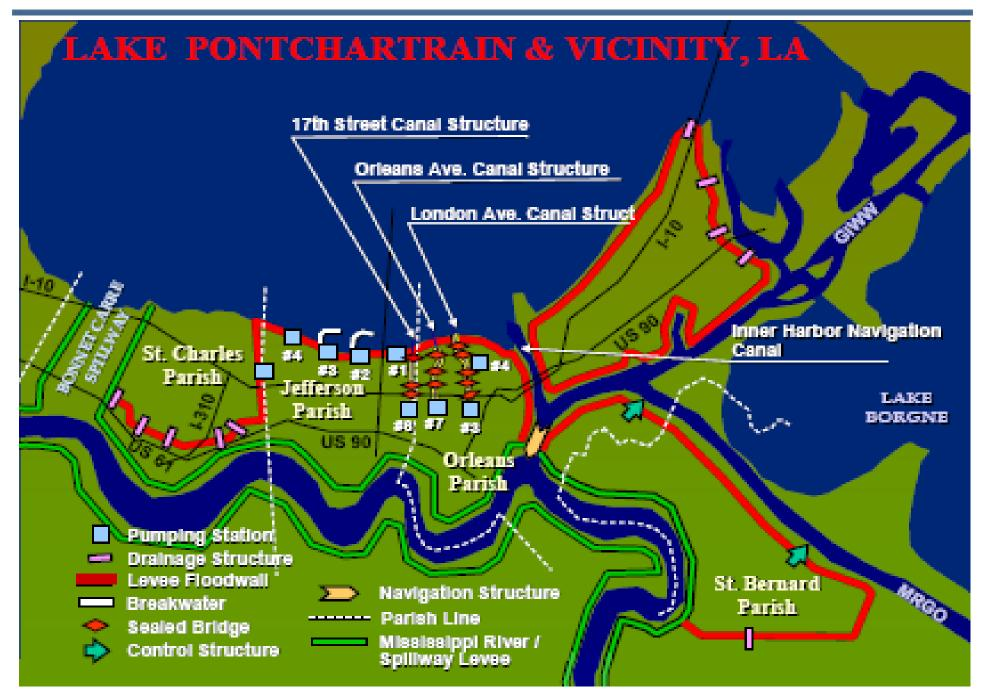
Figure 4. Map showing detailed geometry and features of the New Orleans metropolitan area
