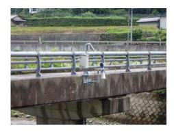
Crisis-management type water gauge (low-cost water gauge specializing in water level monitoring during floods)
