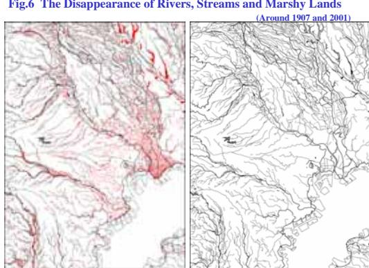
As you can see in this slide, a large number of rivers and waterways have disappeared from the Tokyo metropolitan area in line with the progress of urbanization. The rivers, agricultural waterways and canals marked in red on the diagram on the left have all disappeared, being turned into underground sewers or reclaimed to build roads or other facilities. This is another factor that has increased flood damage.
