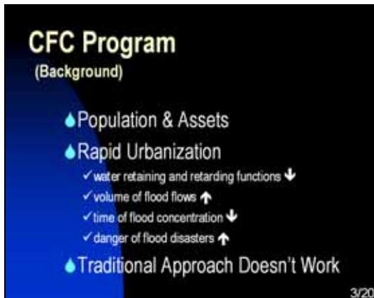
When implementing CFC in Japan, we had to consider that the population and assets are concentrated in the river basins and not in the flood plains. Rapid urbanization occurred in this area, making it difficult to retain and hold water. Therefore, the volume of flood flow increased and flood concentration time decreased, increasing the probability of flooding.
