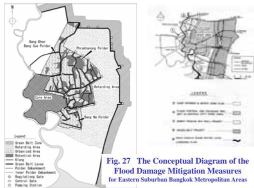
**Fig. 27 The Conceptual Diagram of the Flood Damage Mitigation Measures for Eastern Suburban Bangkok Metropolitan Areas**
