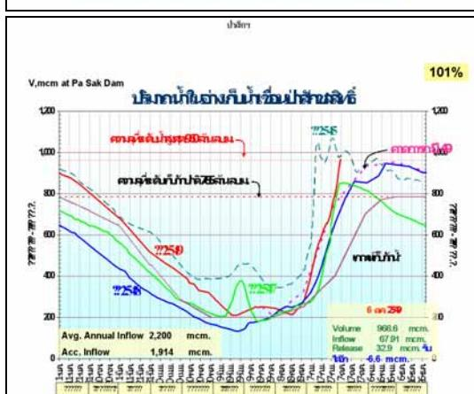
This illustration shows how we try to upgrade Pasak dam for flood control. The water level this dam will be kept low until the end of September. At the beginning of the wet season, we release water to accommodate excess rainwater; since this is a heavy rainfall year, the reservoir is already full.
