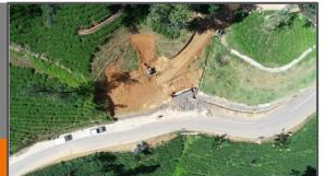
Aerial Photographs obtained from drone surveys are used to generate the contour profiles of sloping terrains
