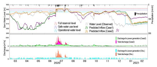
Fig. 3-10 The simulation results of the annual operation of the Oi Hatanagi 1 Dam for the period of March 2020 - February 2021
