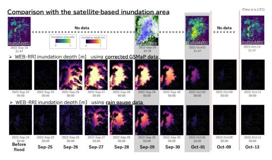
Fig. 3-2 Comparison between satellite-based and RRI-based inundation extent in Kandaba City, the Philippines
