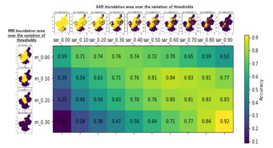
Fig. 3-3 The matching rates of satellite-based and RRI-based inundation extent, calculated using the confusion matrix (the horizontal axis: changes in SAR-based inundation extent, the vertical axis indicating changes in RRI-based inundation extent)
