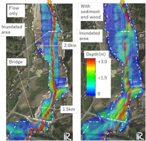
Fig. 3-7 A comparison in the water depth the peak discharge between water only (left) and water with sediment and driftwood (right) (The white dotted line indicates the flooded area interpreted from aerial photos)
