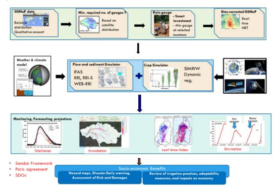
Fig. 3-1 A system for the integrated management of water resources and disasters in poorly gauged basins
