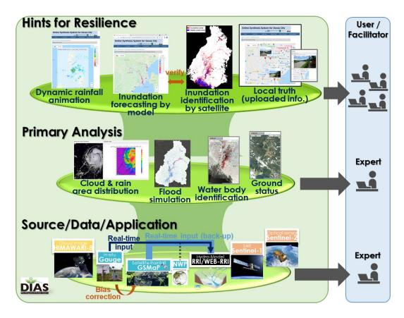
Fig. 3-4 The outline of OSS-SR-based real-time flood monitoring and forecasting
