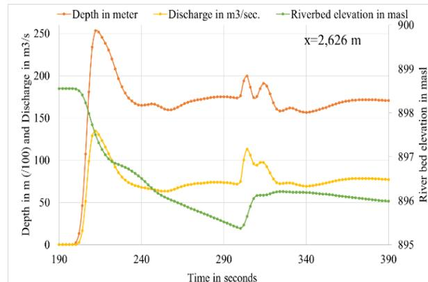
Figure 3 Debris flow characteristic for a return period of 10 years and grain size of 0.1
