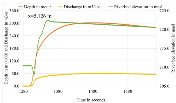
Figure 4 Debris flow characteristic for a return period of 10 years and grain size of 0.1
