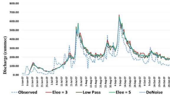
Figure 5: Sensitivity of smoothing of ASTER DEM on discharge at outlet
