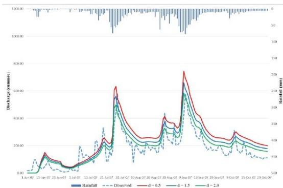
Figure 4: Sensitivity of soil depth values on discharge at outlet for ASTER DEM
