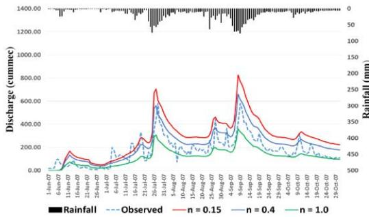
Figure 3: Sensitivity of Manning's n values on discharge at outlet for ASTER DEM
