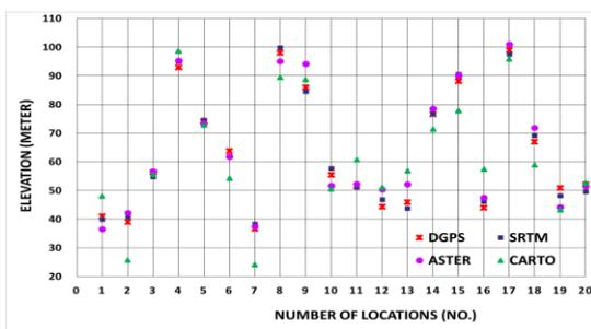
Figure 2: Comparison of elevation of DGPS points with elevation of SRTM, ASTER and CARTO DEM for flood plain
