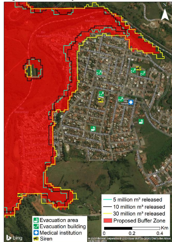
Figure 8. Buffer Zone and affected areas depending on different volume of tailings released
